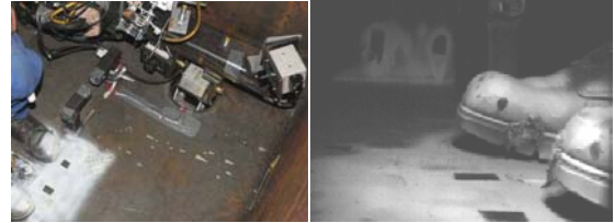
Figure 4 the high-speed camera set-up and view at floor plate
