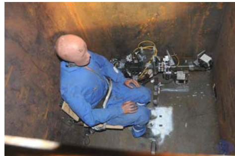
Figure 5 Position of Hybrid III crash dummy at seat system in the test object
